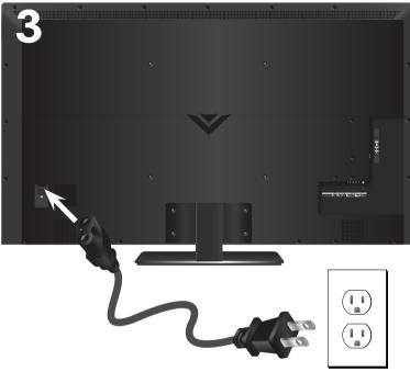
Remove the battery cover by pressing gently on the V logo and sliding away from the remote. Insert the included batteries. Gently slide the battery cover back into place. Connect the power cord to the back of the TV. The flat edge of the connector goes toward the outside of the TV.
